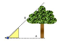
A surveyor estimates the height of a tall tree by measuring the distance from the base of the tree to her transit level with a tape (marked as distance "A" on the diagram), and measuring the angle  $\theta$  required to point the level at the top of the tree (this angle shown as the yellow triangle).
