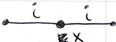
the current  $i$  flowing into and out of node  $x$  is the same.
