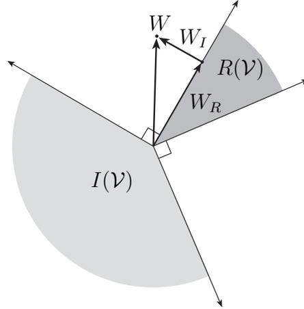
FIGURE 6. The infinitesimal motions  $I(\mathcal{V})$  and the resolvable motions  $R(\mathcal{V})$  of  $\mathcal{V}$  form dual convex cones. Hence, although these are not orthogonal subspaces of  $\mathbb{R}^{3V}$ , a similar decomposition property holds true: any vector  $W$  may be written uniquely as a sum of a vector  $W_I \in I(\mathcal{V})$  and a vector  $W_R \in R(\mathcal{V})$ .
